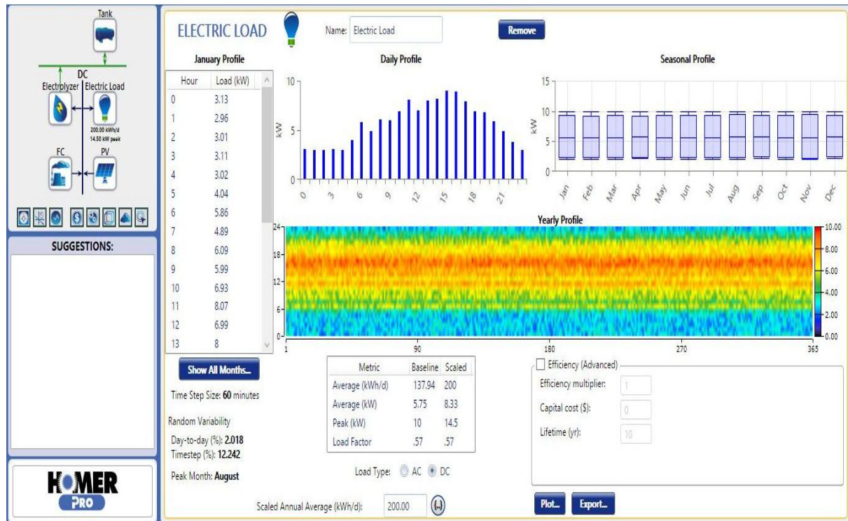
Fig. 6. Microgrid development using HOMER Pro
