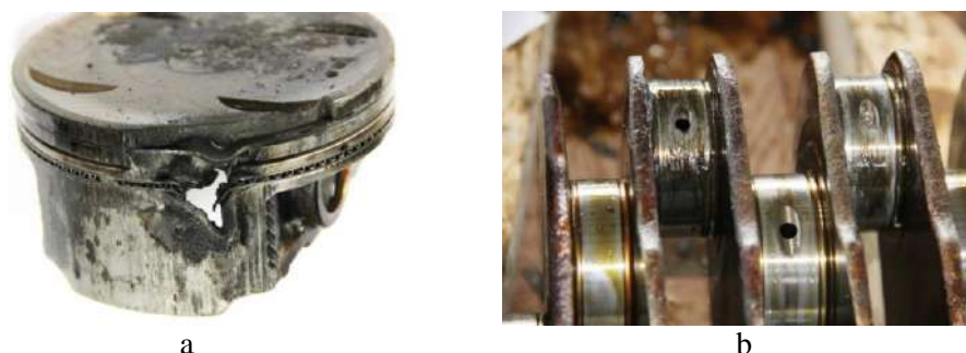
Fig. 5. An example of Subaru automotive engine failure during extremely long inappropriate use on an aircraft: a – burnout of a worn piston; b – destruction of worn crankshaft bearings.
